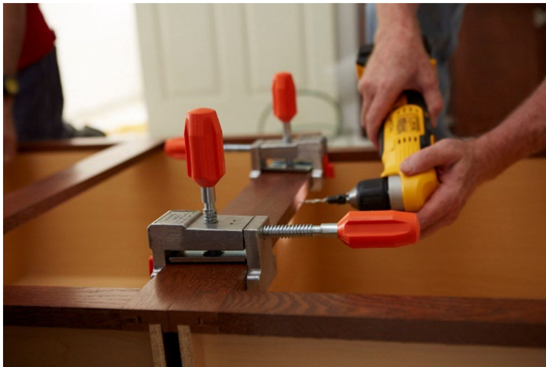
Figure 13-6. Drilling Pilot Holes
