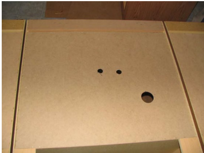
Figure 13-11. Plumbing Cutouts Using a Hole Saw
